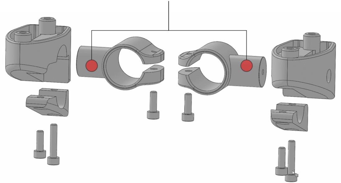
The arm rest position can be adjusted using different mounting holes
