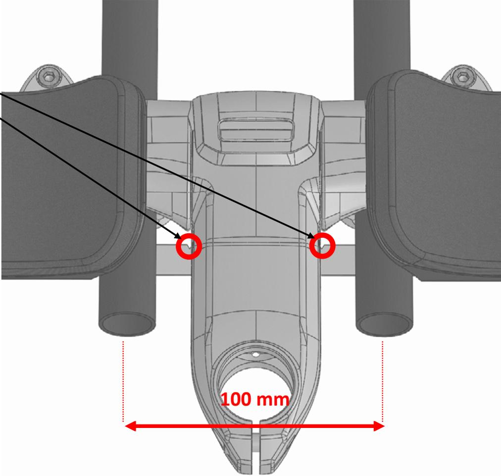
Please note that there is a gap in the clamp when correctly tightened (5 Nm).
